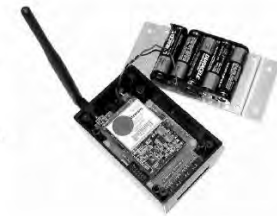
Description and packaging of the WiMMS node proposed by Lynch et al. (2003)
